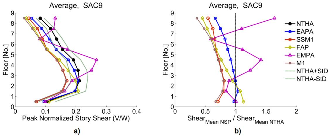
Fig. 9. a) The mean peak normalized story shear profiles and b) the peak story shear error profiles for SAC9
