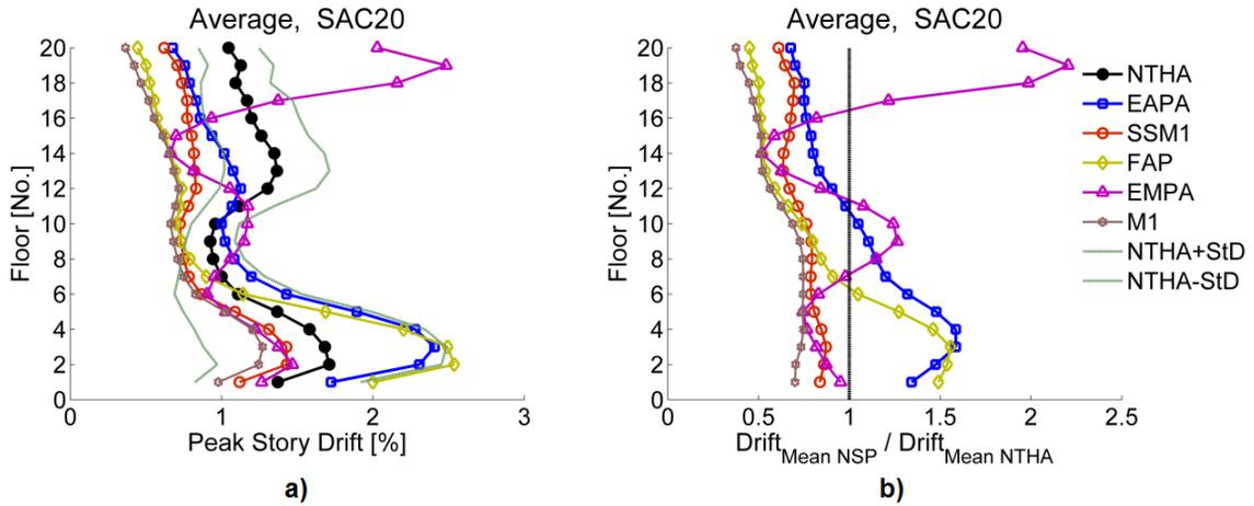
Fig. 12. a) The mean peak story drift profiles and b) the mean peak story drift error profiles for SAC20
