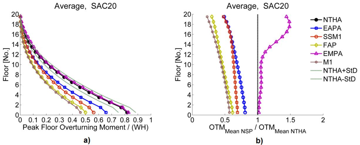
Fig. 14. a) The mean peak normalized floor overturning moment profiles and b) the mean peak floor overturning moment error profiles for SAC20
