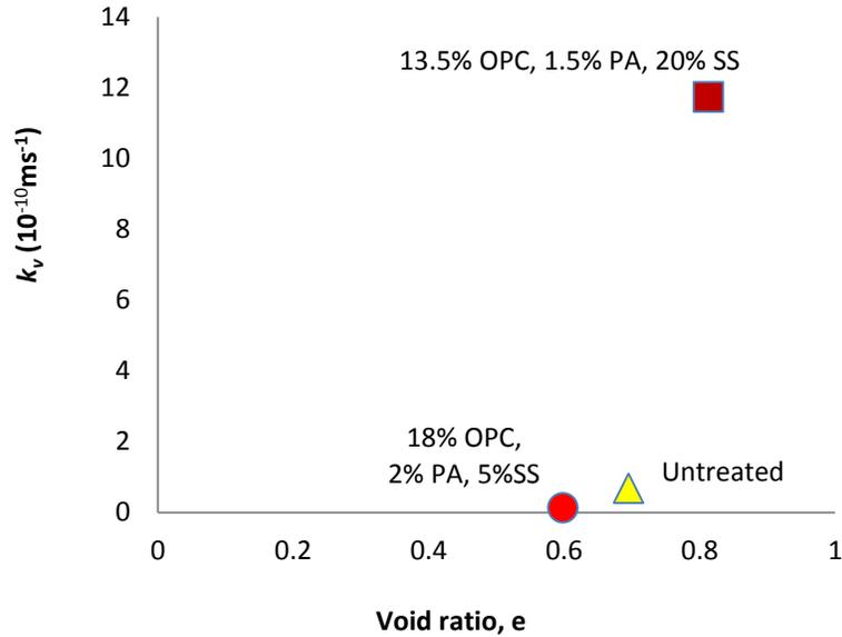
Fig. 7. Permeability-void ratio relationships under 1D consolidation tests
