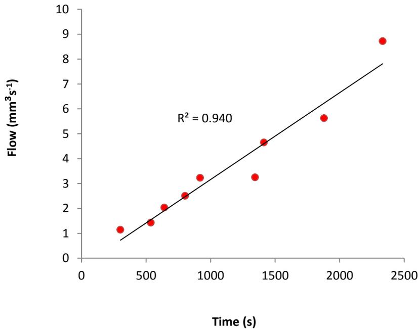
Fig. 4. Flow-time relationship of the untreated clay
