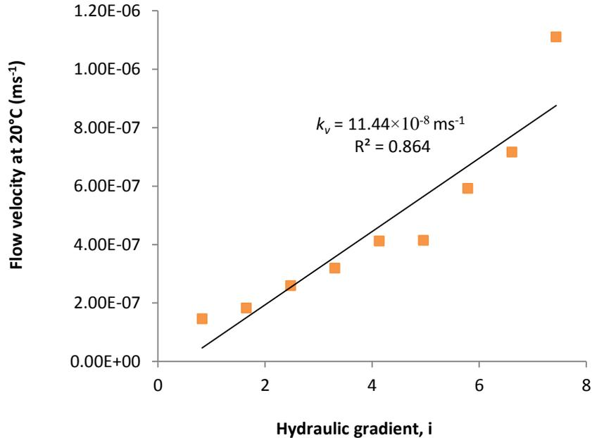
Fig. 3. Rate of permeability of the untreated clay
