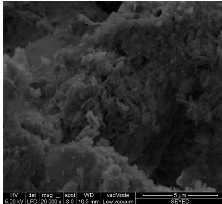
**Fig. 9.** Cementation crystals of the stabilized soil specimen with 18% OPC, 2% PA, and 5% SS after 24 h
