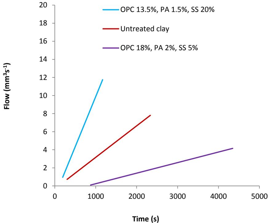
Fig. 6. Flow-time relationships of untreated and stabilized clay
