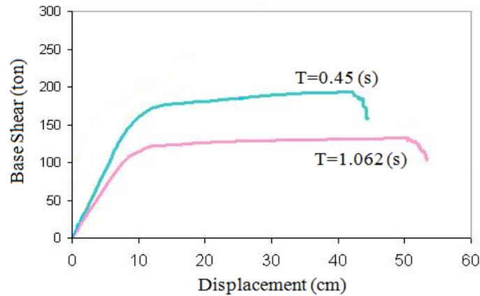
Fig. 2. Static non-linear behavior of the models
