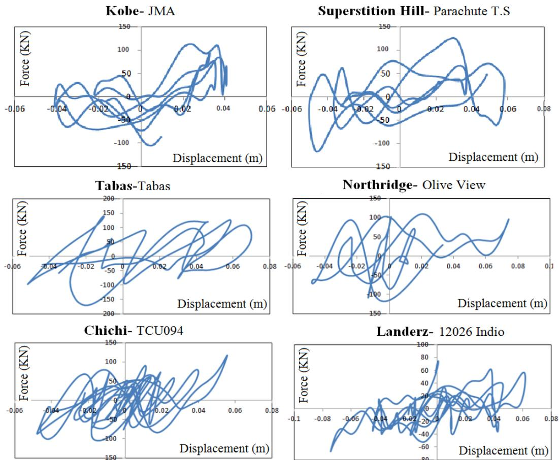
Fig. 3. Hysteresis diagrams for displacement of the node located in the beam to column connection point in story 1, subjected to the four near-fault and two far-fault ground motions based on the scale factor of 1
