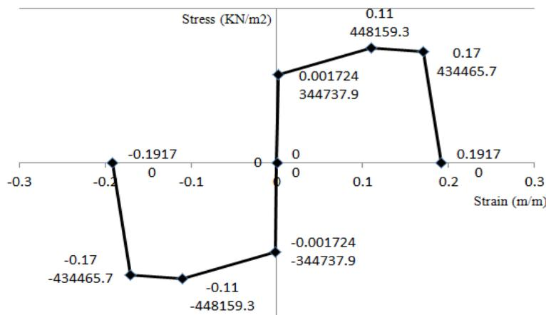
**Fig. 1.** Non-linear behavior of material used for nonlinear modeling
