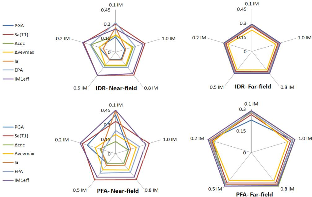
Fig. 6. The coefficient of variation of IDR and PFA subjected to near and far-fault ground motions for a model by the period of 0.45 (s)
