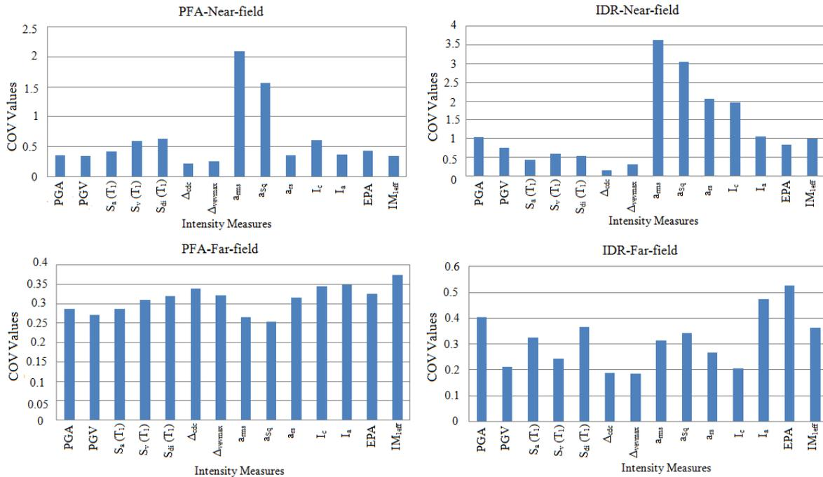
Fig. 5. The amounts of dispersion of structural responses for scaling level of unite subjected to near and far-fault ground motions for a model by period of 1.062 (s)
