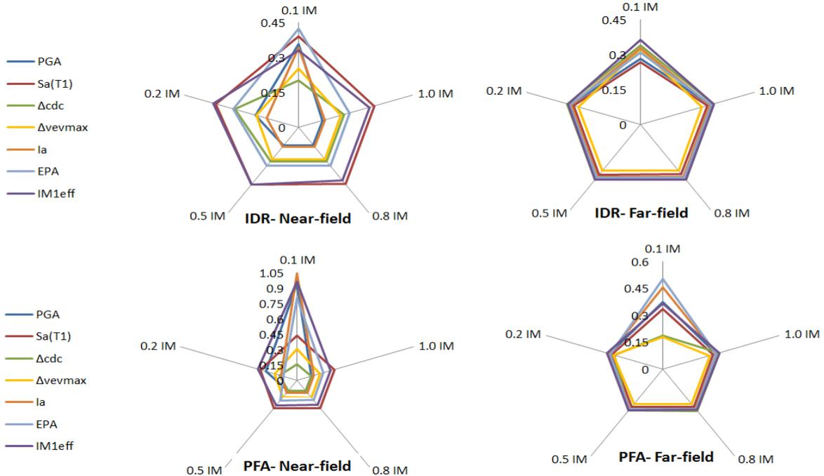
**Fig. 7.** The coefficient of variation of IDR and PFA subjected to near and far-fault ground motions for a model by the period of 1.062 (s)
