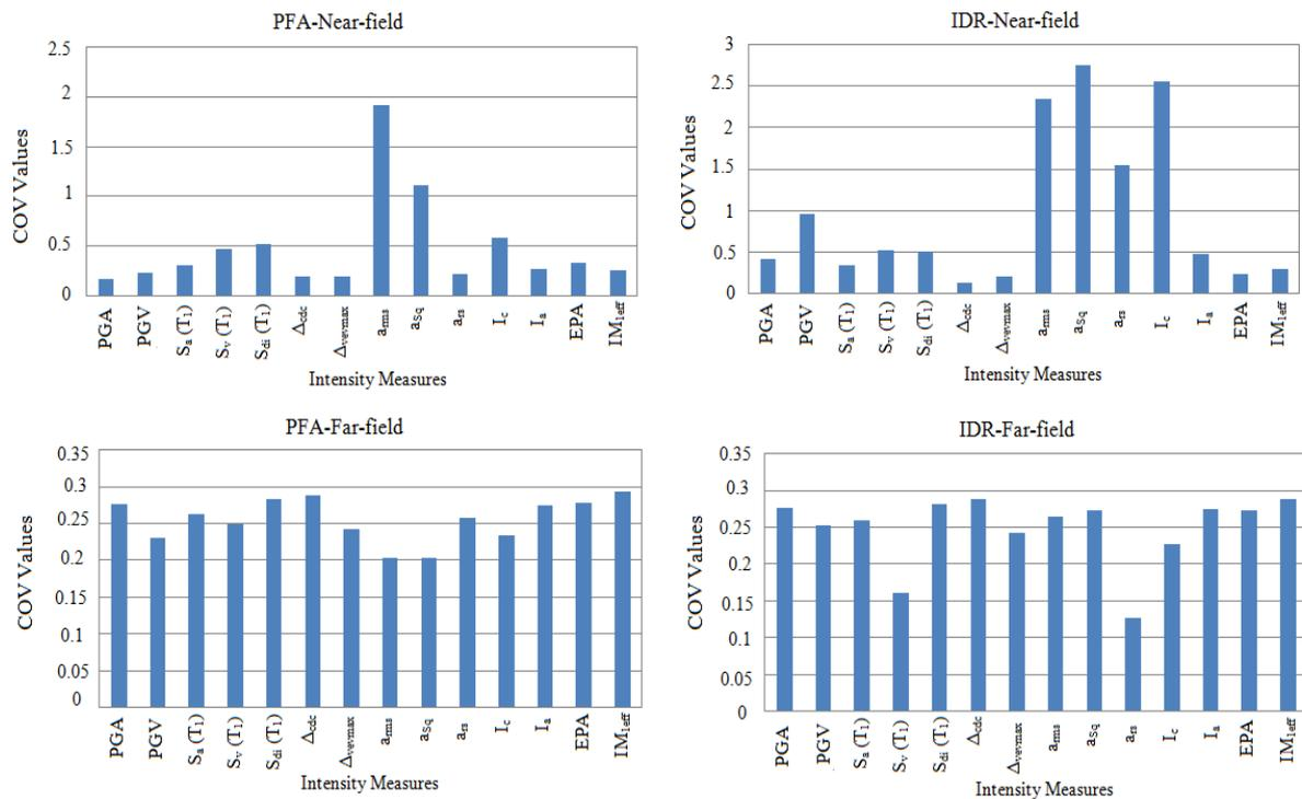
**Fig. 4.** The amounts of dispersion of structural responses for scaling level of unite subjected to near and far-fault ground motions for a model by period of 0.45 (s)
