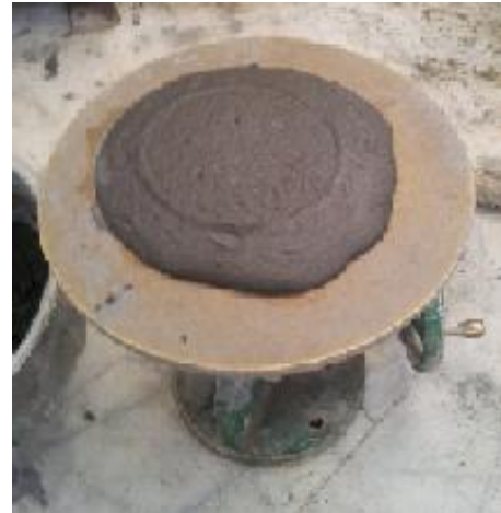
Fig. 3. Flow table test.
