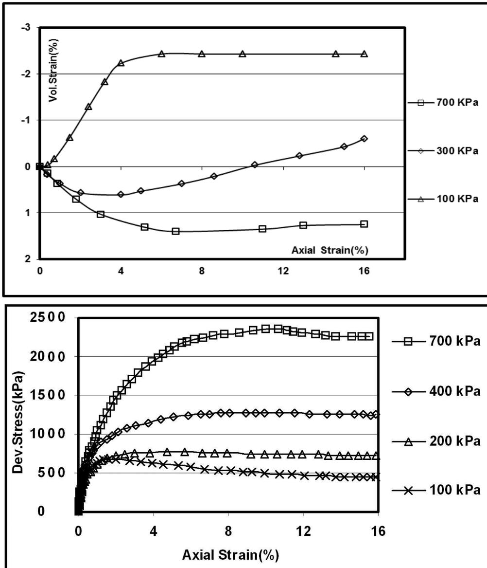
Fig. 10. Variations of deviatoric stress and volumetric strain versus axial strain for V4395 in triaxial test with different confining stresses.
