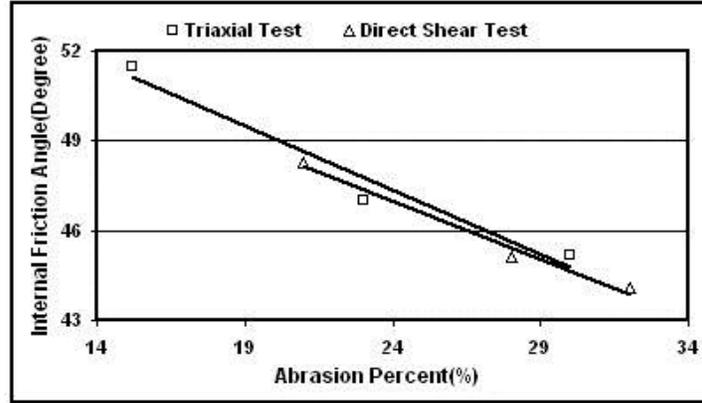
Fig. 11. Variations of internal friction angle versus Los Angeles Abrasion Value for rockfill material.
