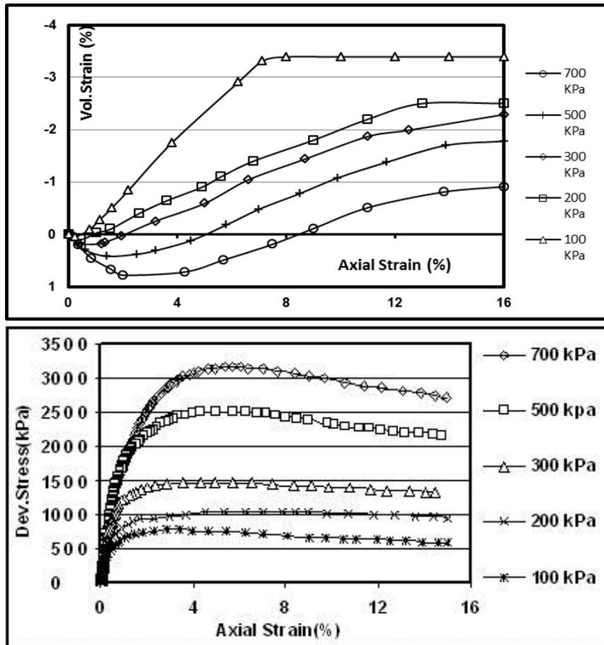
Fig. 8. Variations of deviatoric stress and volumetric strain versus axial strain for I4395 in triaxial test with different confining stresses.
