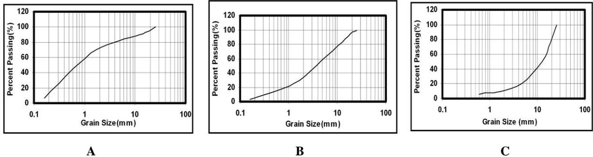
**Fig. 1.** Gradation curve for employed material in Madani and Mianeh dams
