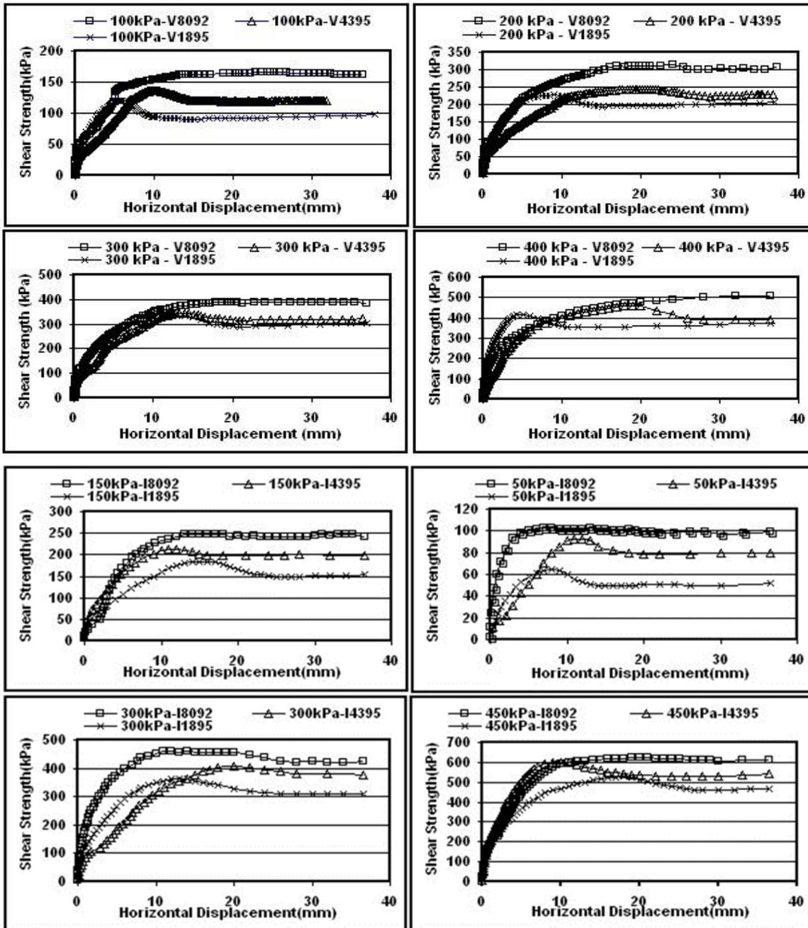
Fig. 6. Variations of shear stress versus horizontal displacement for the rockfill material with different gradations and surcharges in the Mianeh material.
