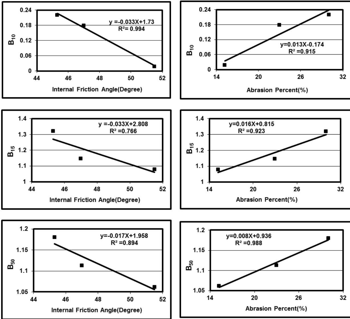
Fig. 12. Variations of different indices for particle breakage with Los Angeles Abrasion and internal friction angle in direct shear test.
