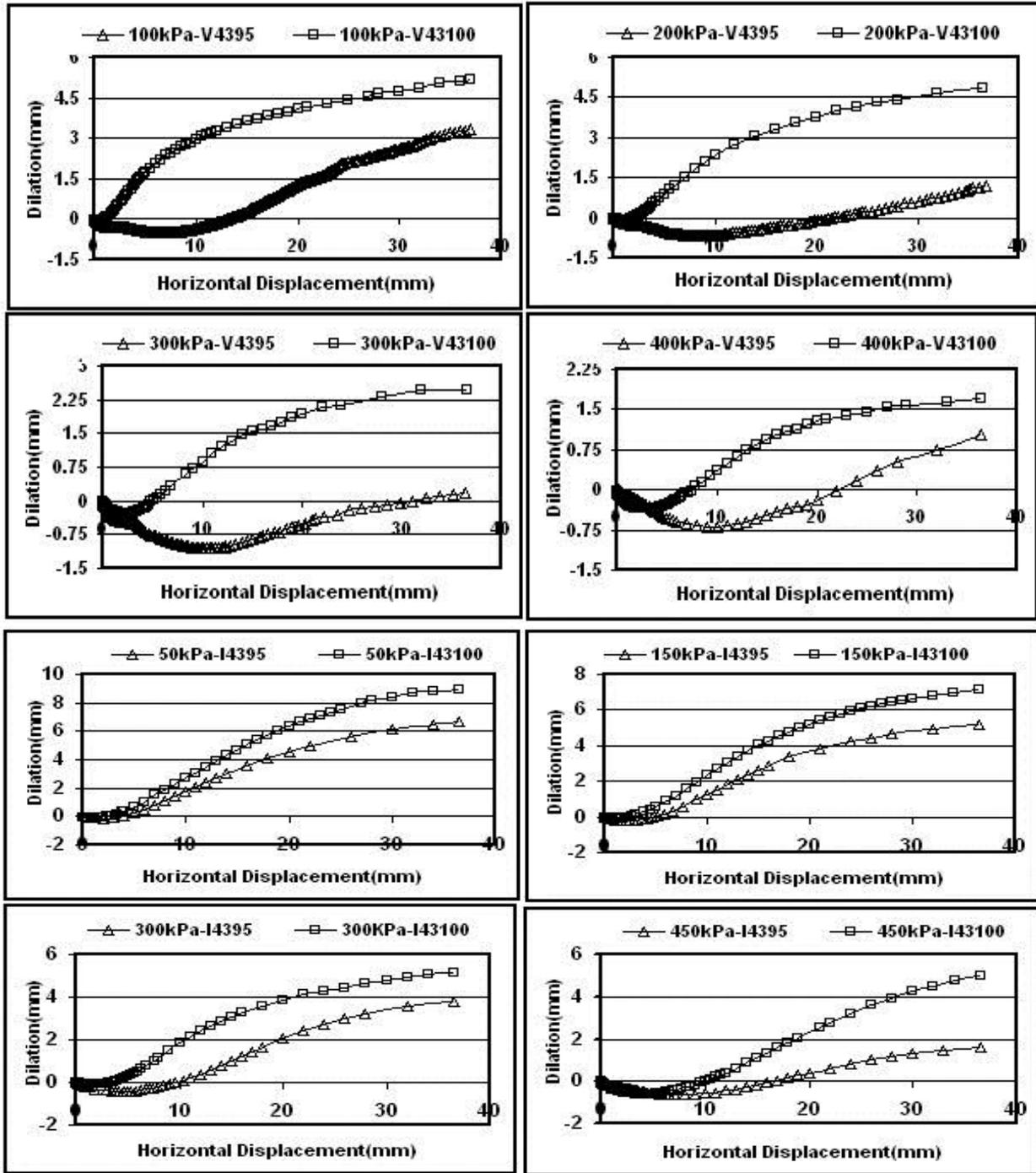
Fig. 5. Variations of vertical deformation versus shear displacement for different levels of compaction and surcharge in direct shear of the Madani and Mianeh material.
