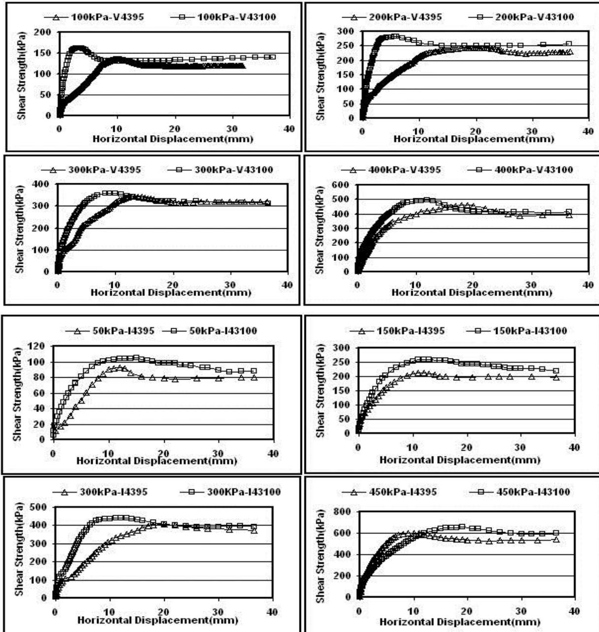
Fig. 4. Variations of shear stress versus shear displacement for different levels of compaction and surcharge in direct shear of the Madani and Mianeh material.
