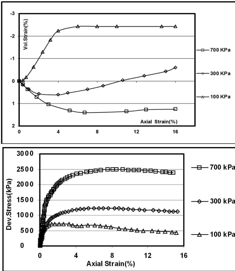
Fig. 9. Variations of deviatoric stress and volumetric strain versus axial strain for I1895 in triaxial test with different confining stresses.
