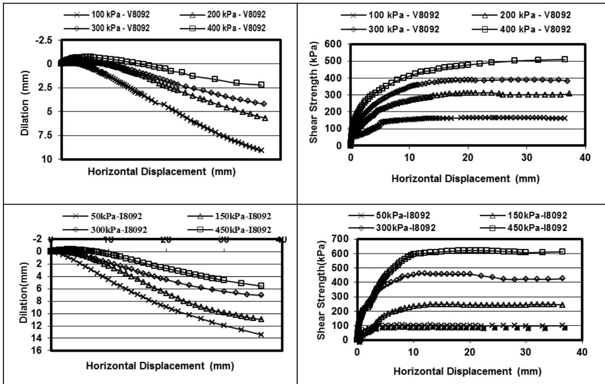
Fig. 3. Variations of shear stress versus horizontal deformation and vertical deformation versus horizontal deformation in direct shear for V8092 and I8092 specimens.
