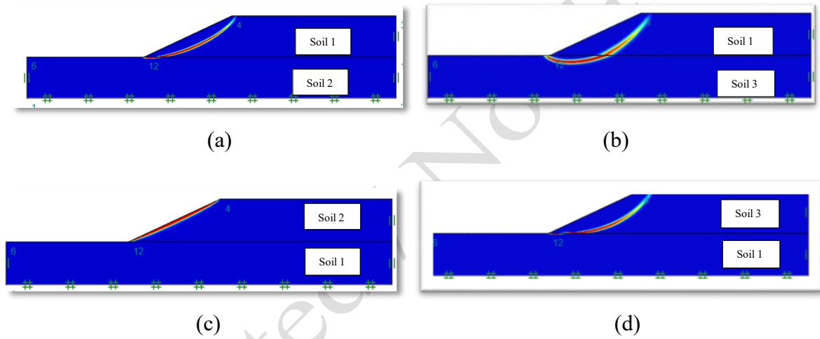
Figure 2: Shear dissipation pattern with fixed top layer (a), (b) and bottom layer (c), (d) for T/D = 0.5 at soil slope 25^\circ .
