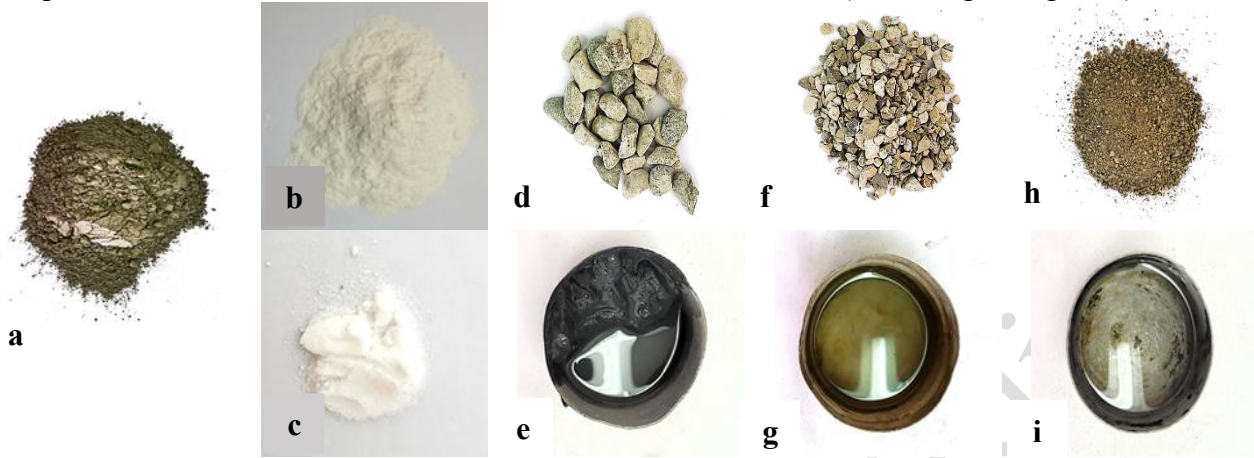
Fig. 3. Materials used in self-compacting concrete mixing plan: a) Cement b) Limestone powder c) VMA d) Almond coarse aggregate e) nanosilica f) Pea gravel g) Super lubricant h) Washed sand i) Water
