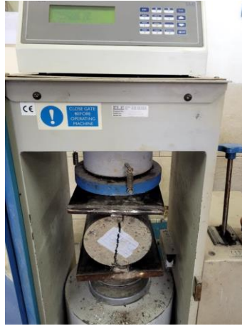
Fig. 5. Tensile strength test on a cylindrical sample
