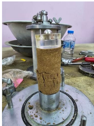
Fig. 10. (a-c) UCS device, (b) untreated soil, (c) treated soil.
