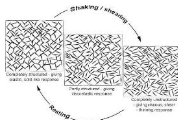
Fig.11. Degradation and reconstruction of a 3D thixotropic structure (Barnes, 1997)
