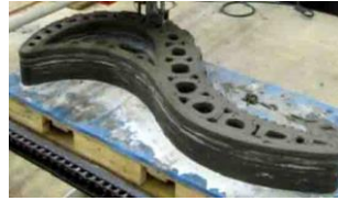
Fig.5. A concrete printed object, highlighting the ribbing on the side resulting from the layered construction technique (Le et al., 2012b)
