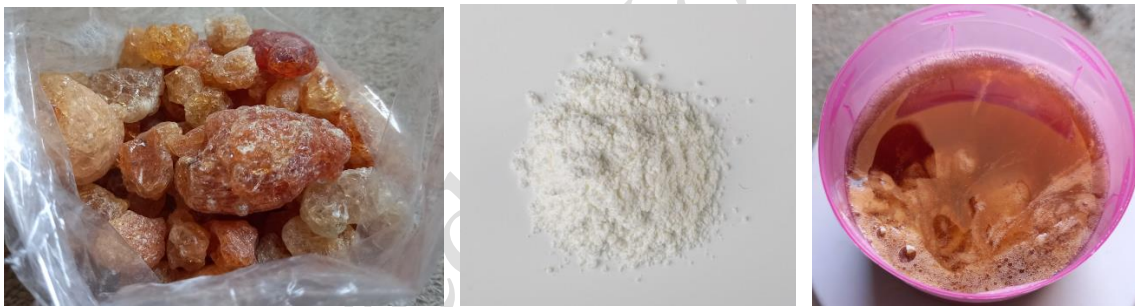
Fig. 2 Gum Arabic: (a) actual, (b) after grinding, (c) extract
