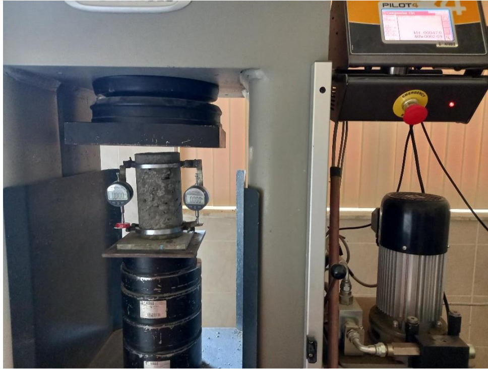
Fig. 7 Test procedure for measuring compressive stress-strain relationship
