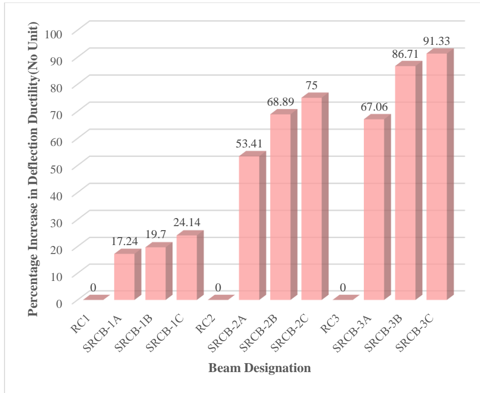
Fig 17. Variation in Deflection Ductility of Rubberized concrete Beams with and without Steel Fibre
