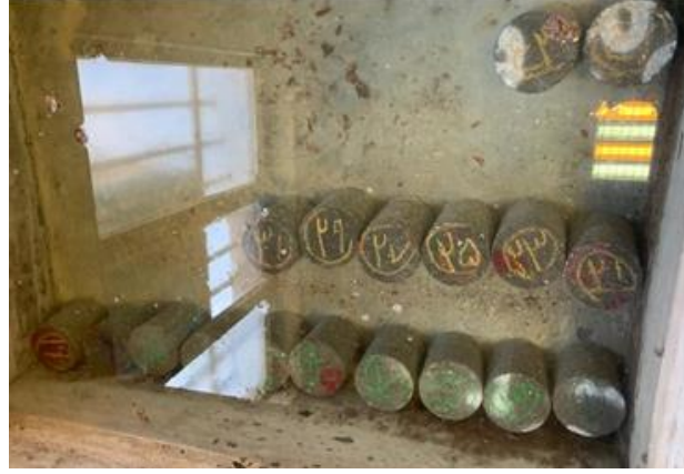
Fig. 3 Curing the 28-day specimens under moisture
