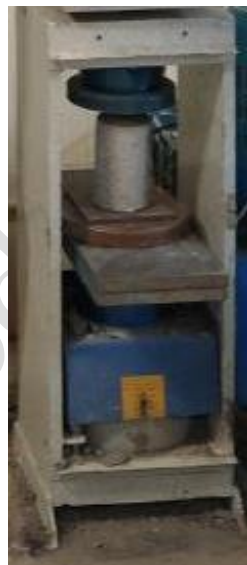
Fig. 2 Compressive testing of samples
