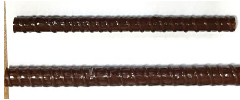
Figure 18. GFRP rebar 8mm and 6mm (closer view)
