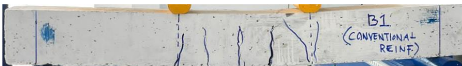
Figure 28. Crack Pattern of Tested (Conventional Reinforcement)
