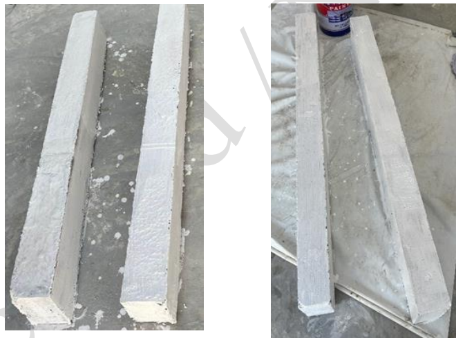
Figure 23. Conventional rebar and GFRP rebar RC beams ready for testing
