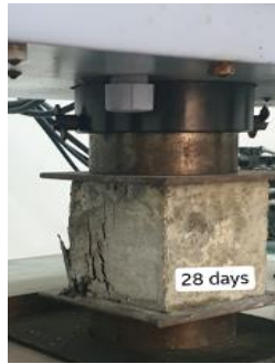
Figure 11. Compressive strength test after 28 days (SCC-SC&SP)
