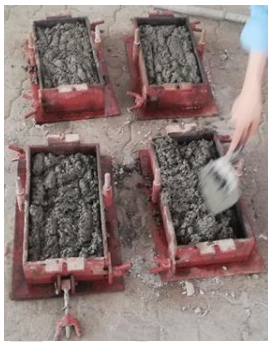
Figure 12. Casting of blocks Figure 13. Finished NC blocks Figure 14. Finished SCC blocks
