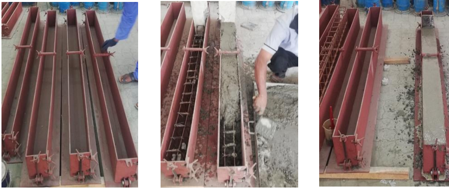
Figure 21. Casting process of conventional rebar and GFRP rebar RC beams
