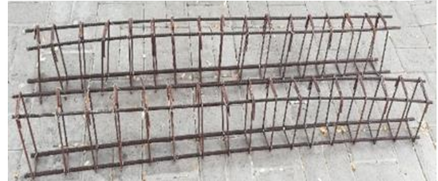
Figure 20. GFRP rebar grill (coloured) (Same cross-sectional area of conventional rebar replaced with GFRP)
