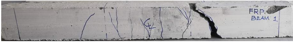
Figure 29. Crack Pattern of Tested (GFRP Rebar)
