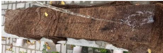
Figure 22. 28-day curing of conventional rebar and GFRP rebar RC Beams
