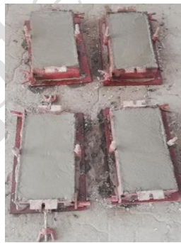
Figure 12. Casting of blocks Figure 13. Finished NC blocks Figure 14. Finished SCC blocks
