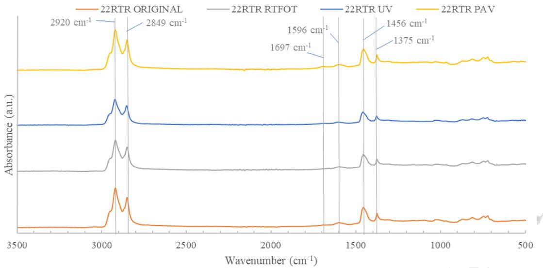
**Fig. 9.** FTIR spectrum of the 22RTR sample
