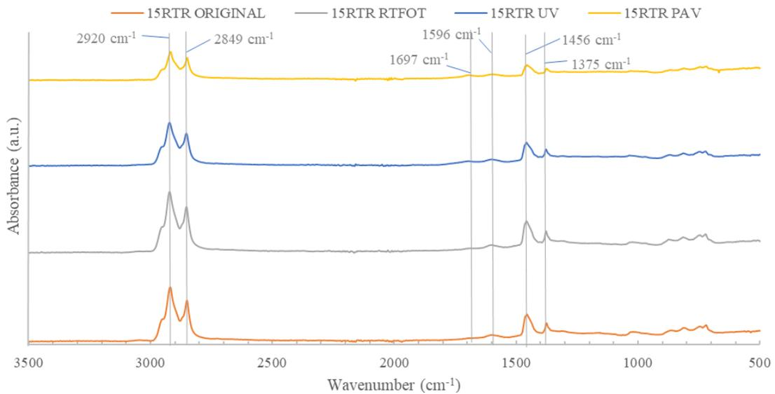
**Fig. 6.** FTIR spectrum of the 15RTR sample
