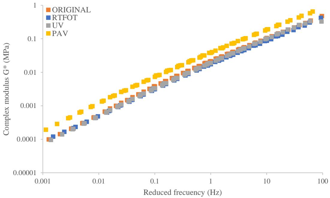
**Fig. 12.** Master curves of Complex Modulus for 15RTR ( $T_{ref} = 55\text{ }^{\circ}\text{C}$ )
