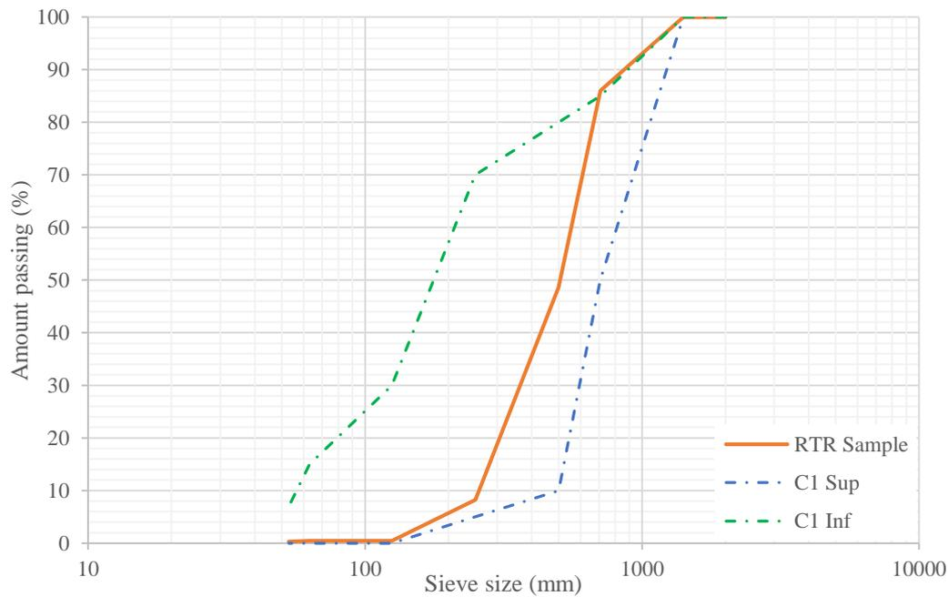
**Fig. 2.** Recycled Tire Rubber granulometric curve
