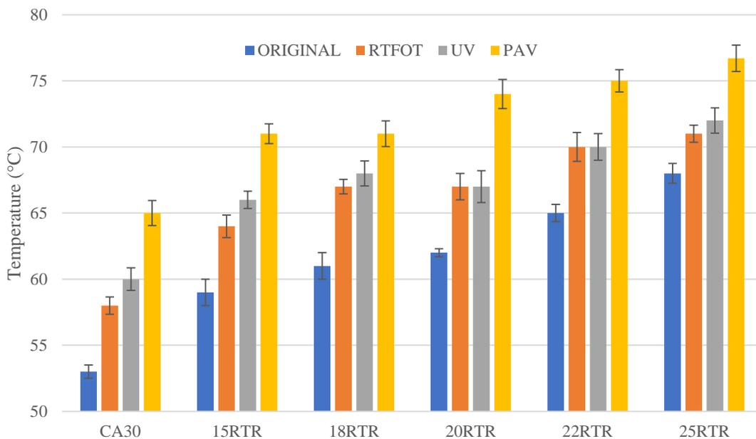
**Fig. 4.** Softening point of the evaluated asphalts
