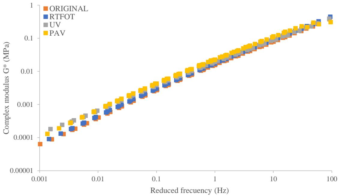
**Fig. 13.** Master curves of Complex Modulus for 18RTR ( $T_{ref} = 55\text{ }^{\circ}\text{C}$ )
