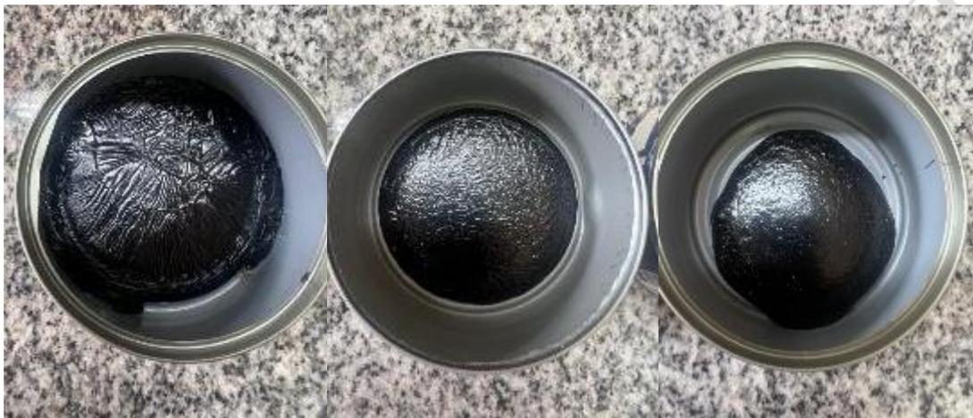
**Fig. 3.** Samples after UV aging. CA30 (left), 20RTR, (center), and 25RTR (right)
