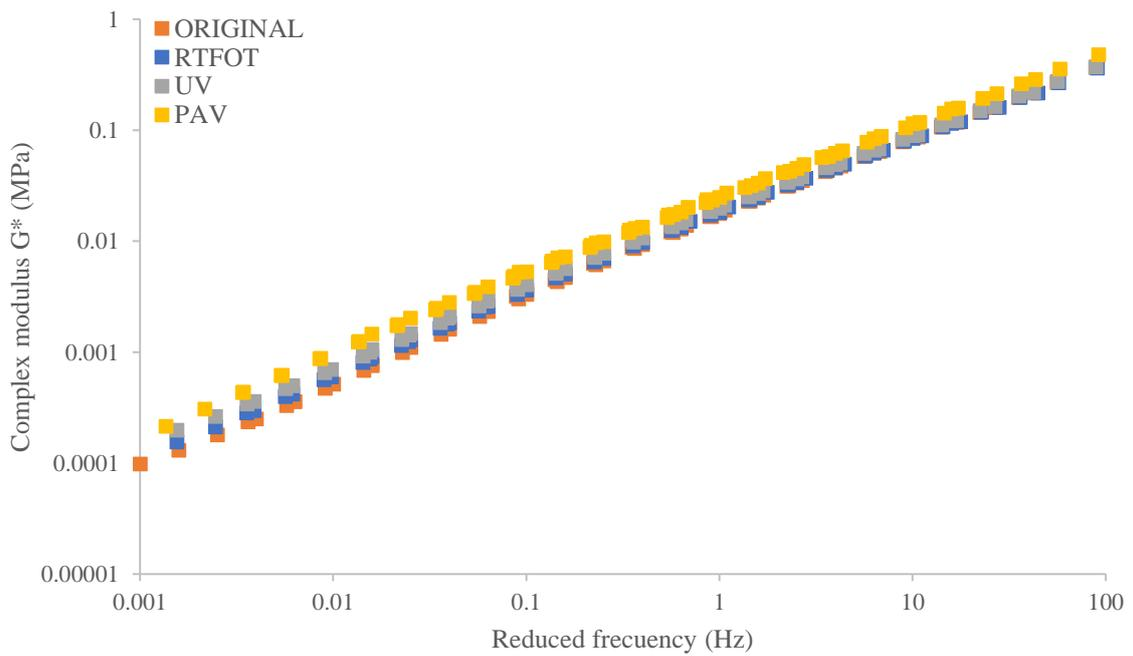
**Fig. 14.** Master curves of Complex Modulus for para 20RTR ( $T_{ref} = 55\text{ }^{\circ}\text{C}$ )
