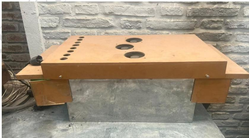
**Fig. 2.** Ultraviolet test chamber
