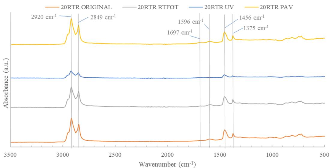
**Fig. 8.** FTIR spectrum of the 20RTR sample
