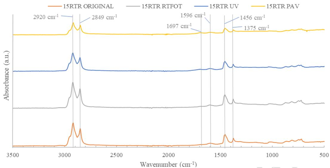
**Fig. 7.** FTIR spectrum of the 15RTR sample
