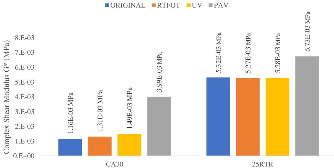
Fig. 17. Complex shear modulus for samples CA30 and 25RTR ( $f=0.1\text{Hz}$ )
