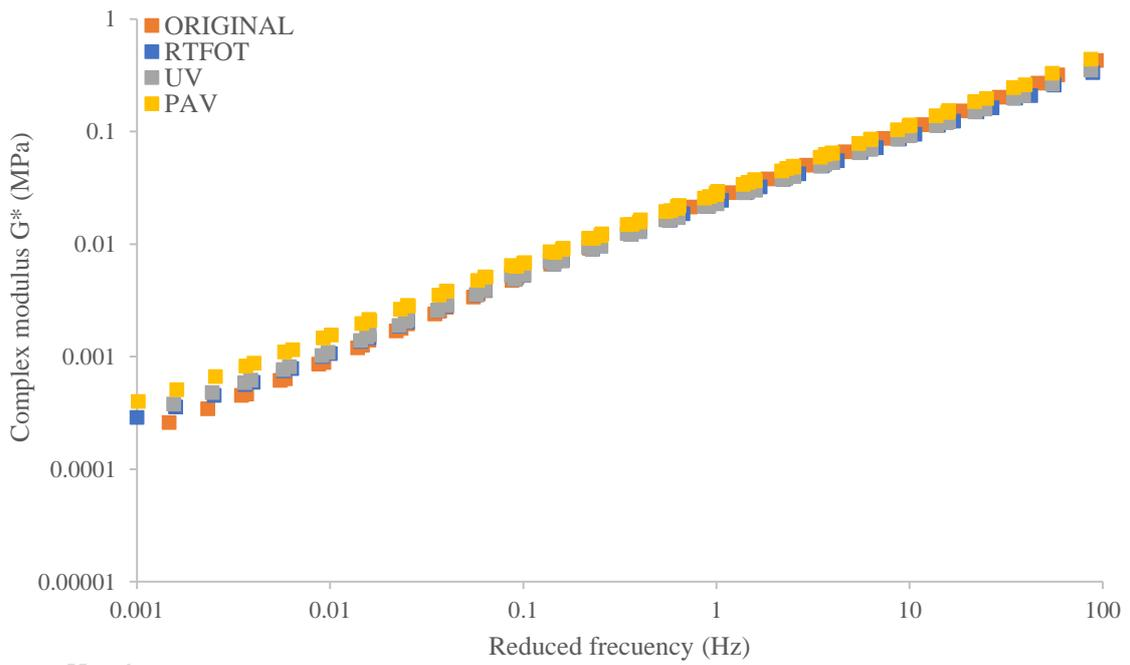
**Fig. 16.** Master curves of Complex Modulus for 25RTR ( $T_{ref} = 55^\circ\text{C}$ )
