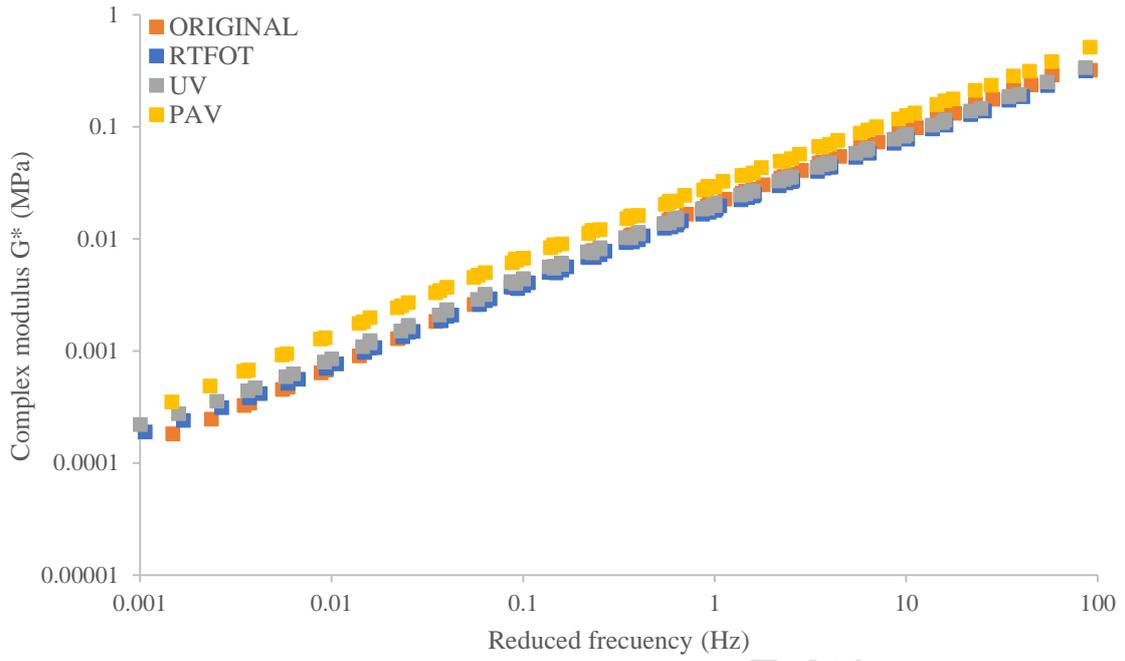
**Fig. 15.** Master curves of Complex Modulus for 22RTR ( $T_{ref} = 55^\circ\text{C}$ )
