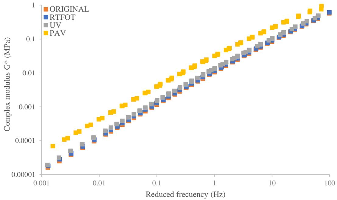
**Fig. 11.** Master curves of Complex Modulus for CA30 ( $T_{ref} = 55\text{ }^{\circ}\text{C}$ )
