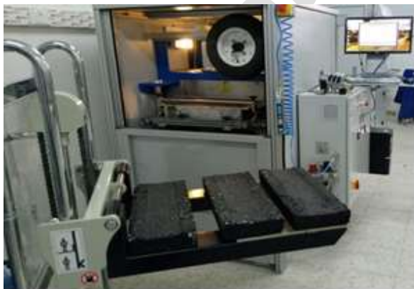
Fig. 6. Rutting test device.
