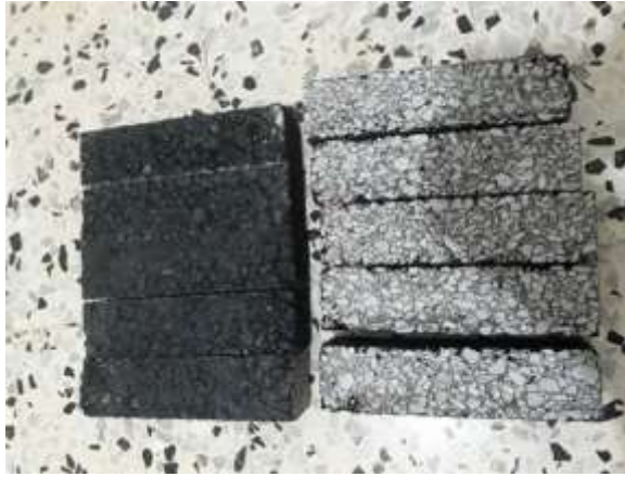
Fig. 4. Prismatic specimens in control and modified bituminous concrete.
