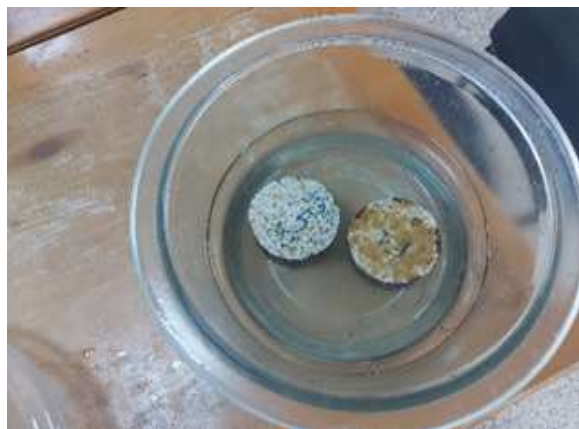
Fig. 7. The leaching test device.
